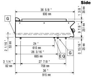
EQ = Equipotential screwG = Gas connection
